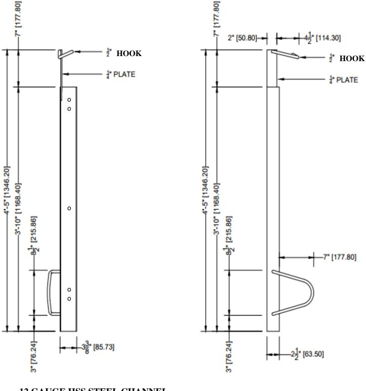
12 GAUGE HSS STEEL CHANNEL 18" O.C. SPACING POWDER COAT BLUE OR GALVANIZED LAG USING 3/16'' (4.763 MM) X 1 3/4'' (44.45 MM) TAP CONS FOUR SECTIONS PER BIKE RACK
